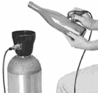
CO2 Tanks measure about 7 inches in diameter by 3-feet in height and weigh 43-pounds full. Tank pressure is in the 800-PSI range. Be sure to follow the supplier's guidelines and safety practices at all times.
