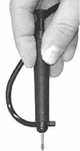
It is a good idea to check how far the bur is inserted into the handpiece when you first receive your tool as this is the correct depth. Do not extend the bur out to increase its reach. If you need a longer bur, please note that our burs come in surgical lengths which are a quarter inch longer than standard burs.
