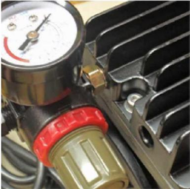
2. When installed properly, the air gauge should be near the top and the brass fitting will be screwed completely in. The air adjustment has been preset to power your high speed handpiece at the correct pressure. To raise or lower the pressure pull out on the adjustment and twist it slowly. Pushing the adjustment valve will lock it into position. We suggest you do not adjust this valve as it is preset for your Turbo Carver.
