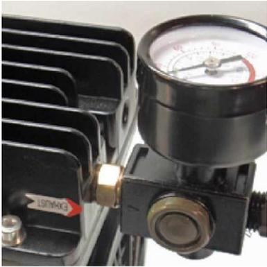
1. First - Connect the Air Gauge Adjustment valve into the EXHAUST PORT. This is the outlet for the air. The other end of the air compressor is the intake port. Prior to installing this valve remove any particles or obstructions that may be in the threaded exhaust or intake ports.
