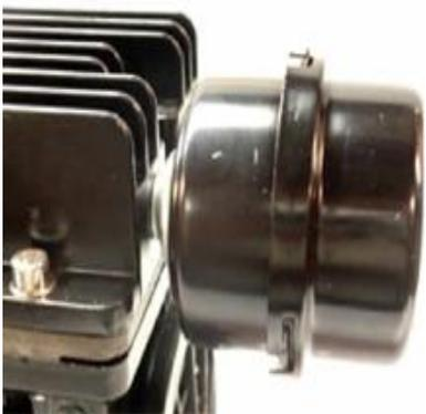
3. Next, hand turn the Air Filter completely into the intake port.
