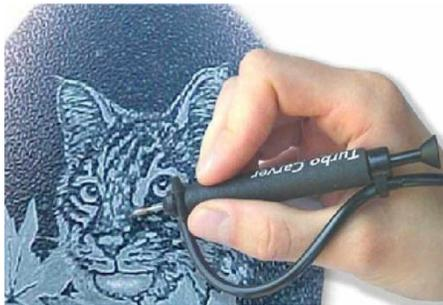
The principal behind the Turbo Carver is angular velocity, not torque. The advantage of high speed air tools lie in their phenomenal ability to precisely remove material without stressing you or what you are working on.
